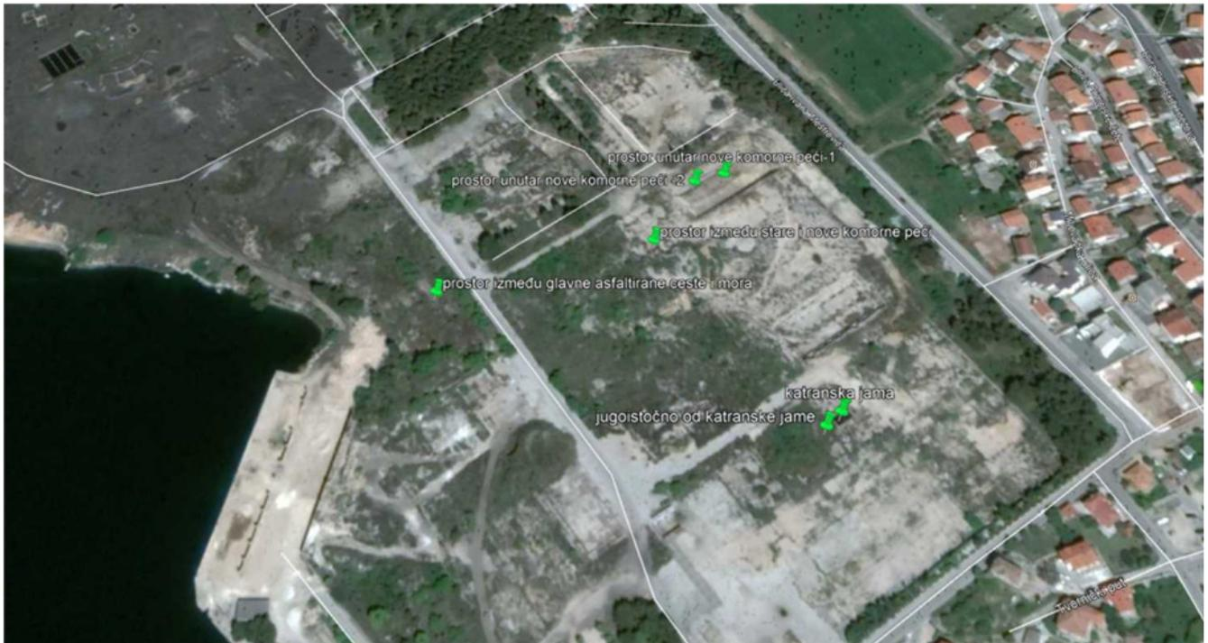
The locations where samples were taken (Picture from the Research plan and report on the remediation of the site of the former TEF d.d., made by Okion d.o.o., May 2018)
